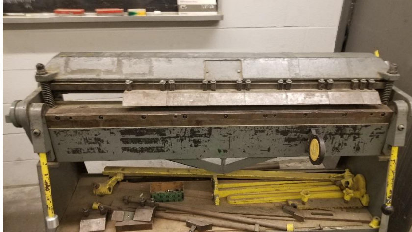
Figure 18: The sheet metal brake to be used - note the sliding "fingers" on the top clamping surface
