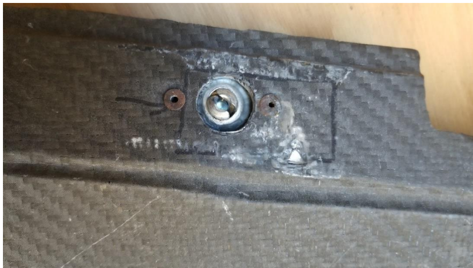
Figure 6: Skewed location of the aluminum insert
